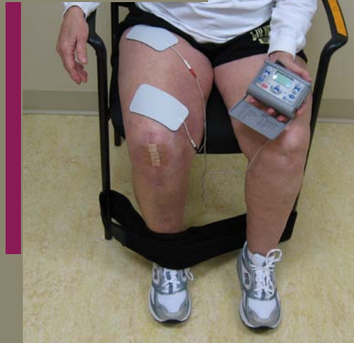
NMES unit fires electrical bursts that force quadriceps to contract.
